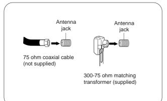
Connect the 75 ohm cable from the combination VHF/UHF antenna to the antenna jack.
